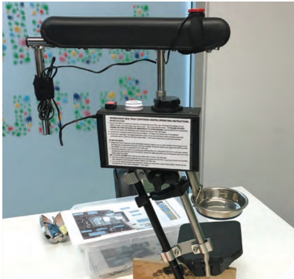
The button version installs the button on the armrest of the wheelchair and the treat falls into a small tray, adjusted to the right height for the dog, without being in the way for general movement of the wheelchair.
