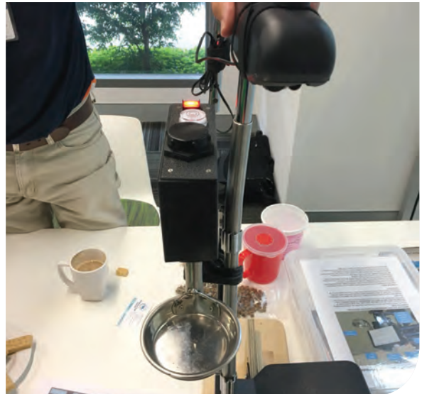
The button version installs the button on the armrest of the wheelchair and the treat falls into a small tray, adjusted to the right height for the dog, without being in the way for general movement of the wheelchair.
